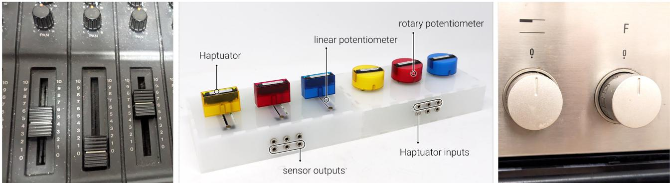
**Figure 3: Middle: Participants explored their rendered vibrotactile effects with two types of physical elements: sliders (left) and knobs (right). Sides: similar UI elements found “in the wild”.**
