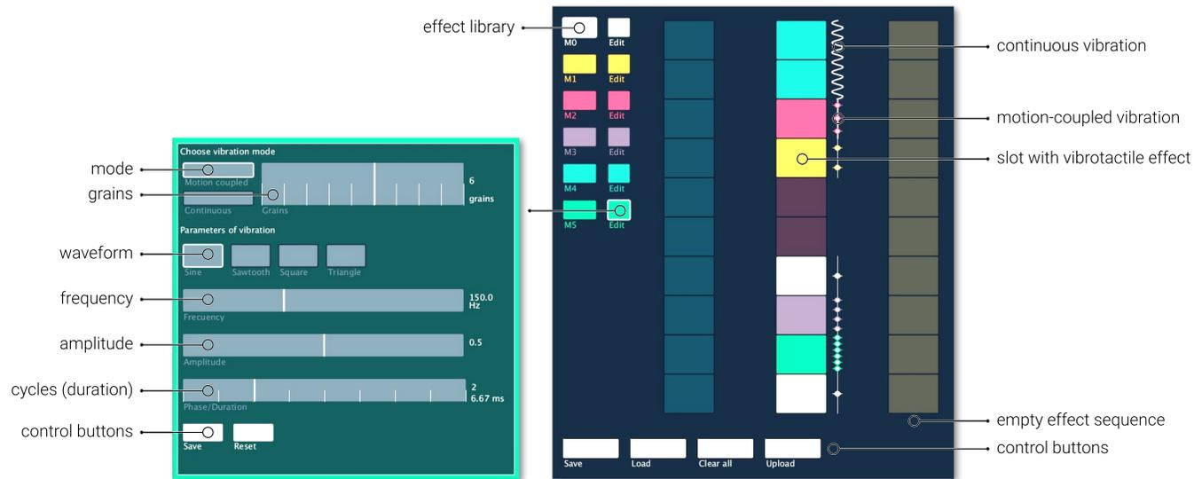
**Figure 2: The GUI used for this study has two windows – one to parameterize vibrotactile effects: *Effect Designer* (left), and another to create sequences of these effects: *Effect Sequencer* (right).**
