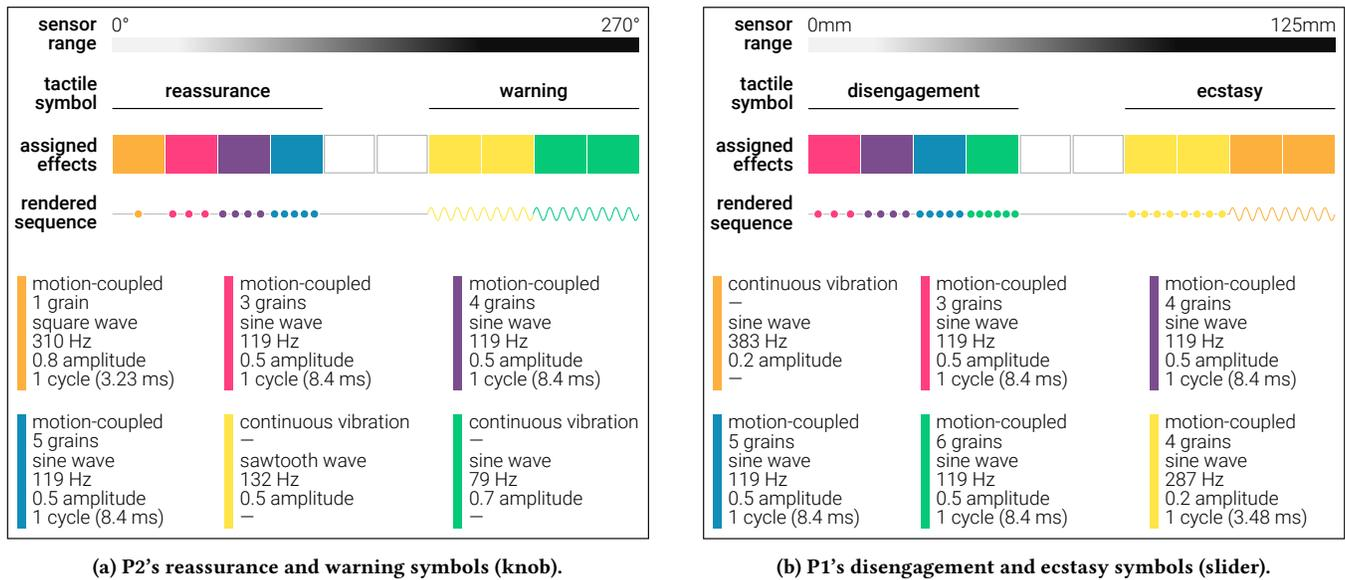
**Figure 5: Example tactile symbols designed by two participants are shown with the rendered sequence and the parameter values for each vibrotactile effects in those rendered sequences.**
