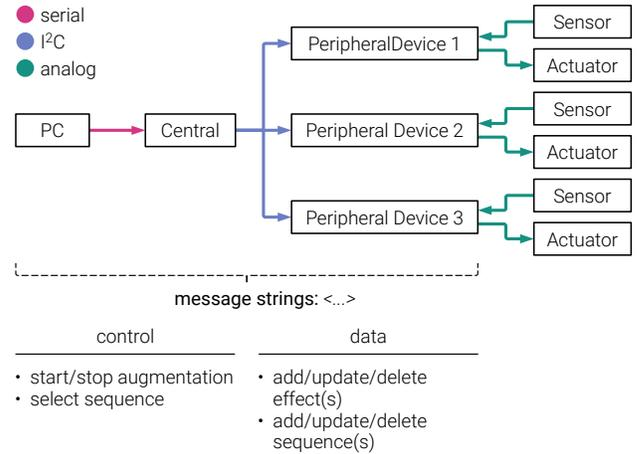
**Figure 4: The PC and the central controller uni-directionally communicate via USB-serial. Each peripheral device is connected to the master using an I2C, and the communication is uni-directional from the central device to the peripheral devices. USB-serial and I2C communication is done with formatted message strings. The messages are used to modify the system’s state (e.g., start/stop augmentation) and transfer data to the peripheral devices (e.g., send effects and effect sequences).**
