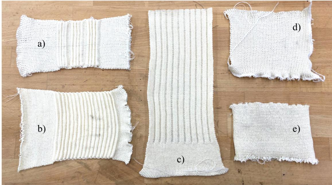
Figure 7.12: Samples of different knit structures for the collar body. Three Milano rib variations (a, b) were compared to a 2x3 rib (c) and two full bed rib stitches (d, e).
