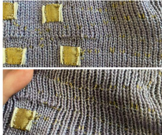
Figure 7.19: The conductive thread stitched along the knit (top). When stretched, the conductive traces stretch with the knit (bottom).
