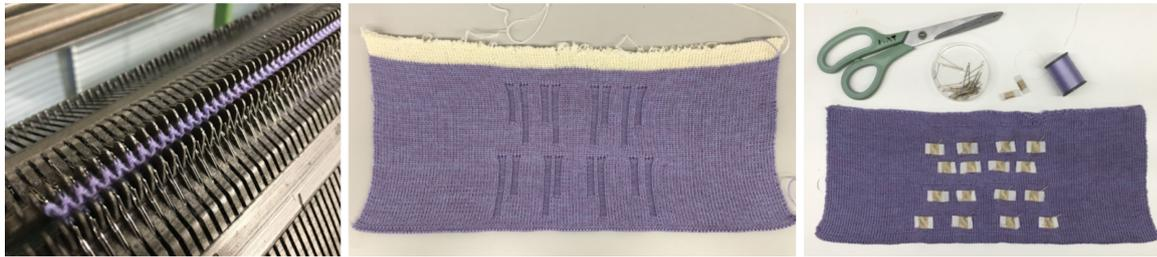
Figure 7.16: Creating the final collar body (left) and attaching the fabric electrodes (right). The final iteration uses the alternated relief stripes to mark the electrode locations externally (middle).
