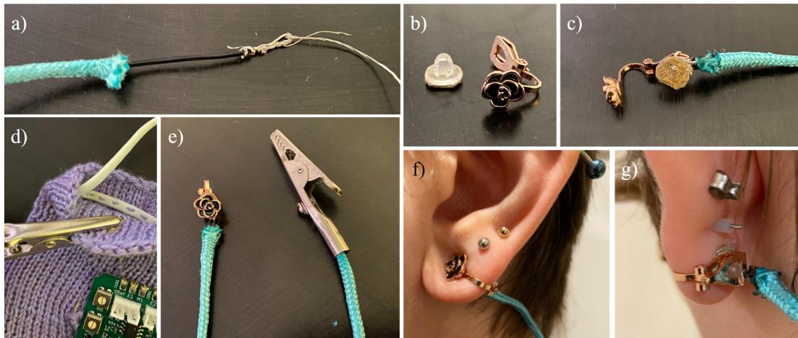
Figure 7.20: The construction of the earring reference electrode, starting with the cabling (a), stitching the conductive fabric to the earring pad (b-c), and securing the electrode to the collar and reference inputs (d) for a complete wearable (e). I wear the electrode along with my normal jewelry (f, g).
